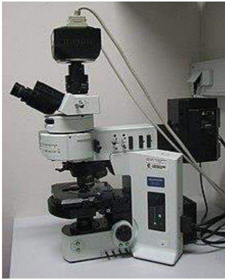
Fig: An upright fluorescence microscope (Olympus BX61) with the fluorescence filter cube the objective lenses, Coupled with a digital camera.
